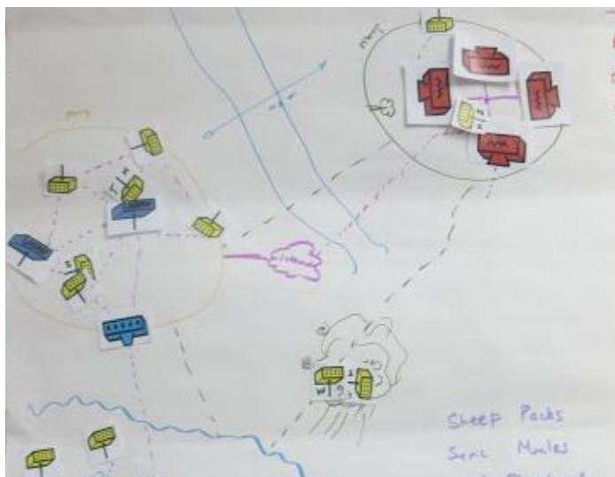
The Janastu network plan incorporates a delay tolerant network to allow for opportunistic data sharing between communities. Their network design consisted of sheep packs, sync mules and good shepherds.
